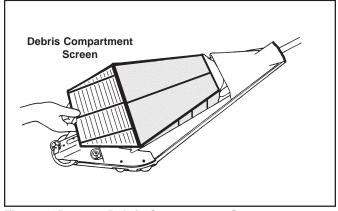
Figure 4. Remove Debris Compartment Screen
